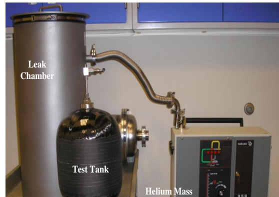
Figure 8: CTD's test bench to measure permeation rate in KIBOKO® tanks using a leak chamber and Helium mass spectrometer.
