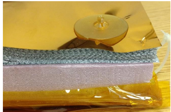
Figure 2. An MLI standoff holding the MLI blanket and foam insulation to the metal surface.
