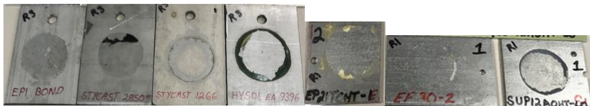
Figure 6. Epoxy failures on stainless steel samples.
